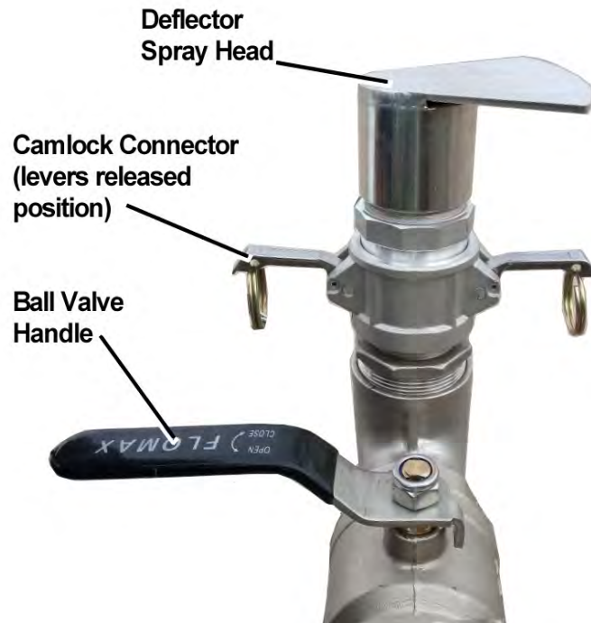
Figure 8 – Water Deflector Spray Head (optional)
